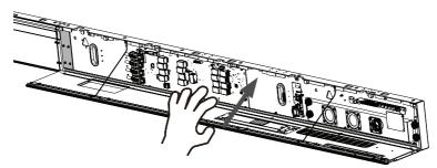
12. Replace the Left Cover by aligning it properly with the System Control Box; then the Left Cover should attach magnetically.
