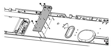
5. Further secure the Connector Plate with the two provided screws (M3 x 5 mm).
