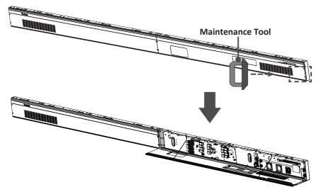
3. Remove the Left Cover by gripping the top edge of the Cover and pulling it toward you. The Left Cover should simply lift away.
