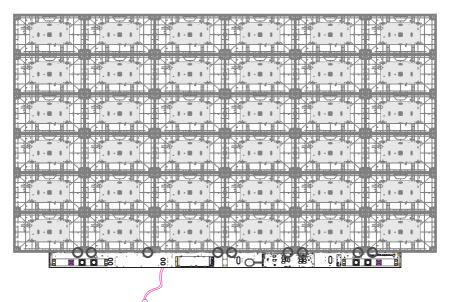
7. Connect the Power and Network Cables of the Cabinets from the System Control Box to each Cabinet. Start from the bottom and move to the top (see Appendix B for example system wiring diagrams, including wire colors and connection points).
