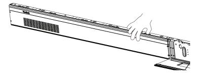
4. Secure the System Control Box panel with the Connector Plate using the provided screws (M3 x 6 mm).
